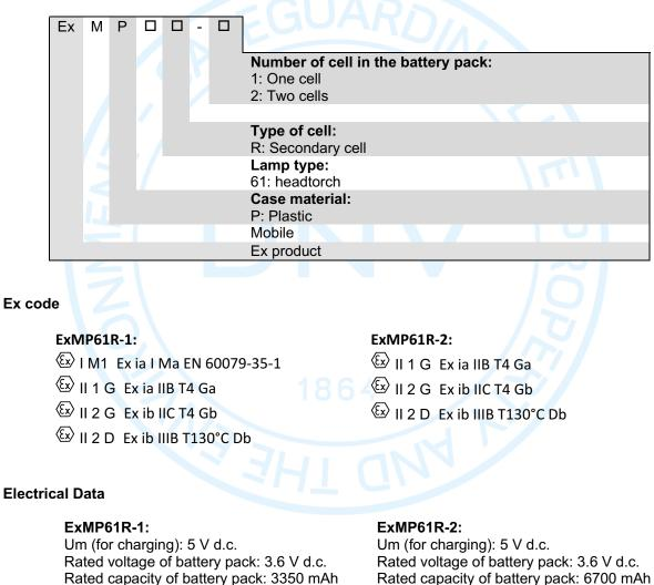
Degrees of protection (IP Code) IP66, IP67 (1 m, 30 min)
